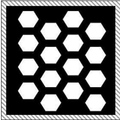
Figure 1: The design of the hexagonal lattice used in RPI's solid state detectors [6].
